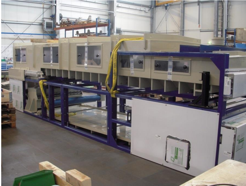
Image 2. BHS Polypropylene belt filter with fume hood built for the filtration, washing, and drying of the sulfuric acid slurry.
