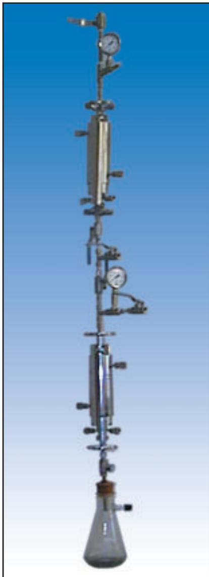
Dual Pocket-Leaf Filters for testing of sequential process operations
