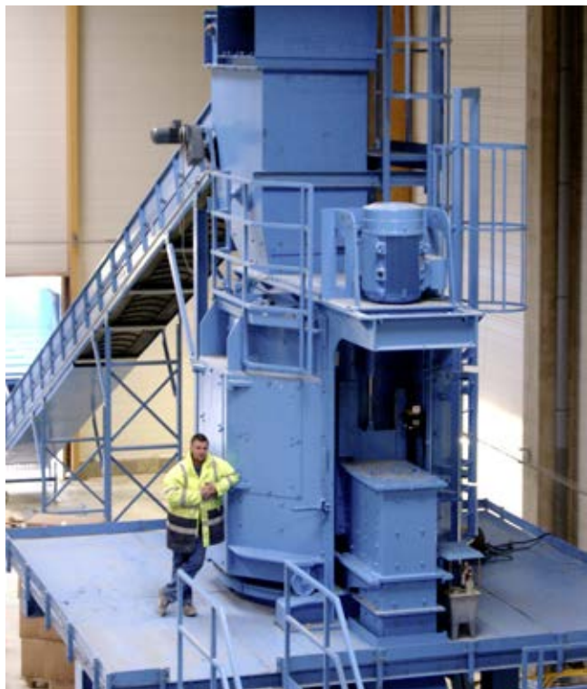
Construction and assembly of a complete BHS recycling plant in France. The E-Scrap plant is equipped with a BHS Rotorshredder of type RS 2018.
