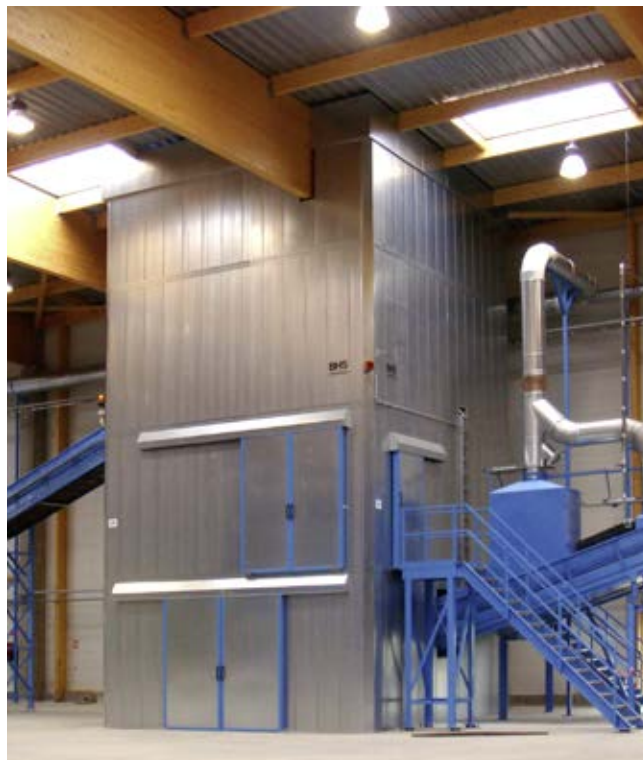
The Rotorshredder is enclosed for disaggregation of E-Scrap in the first recycling stage.
