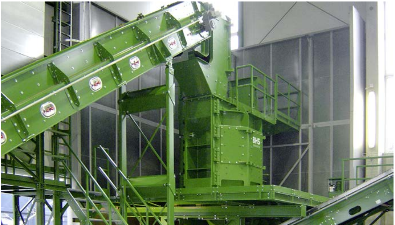
Installation of a complete BHS recycling plant for crushing secondary metals in Austria. The plant is centered on a Rotorshredder from BHS, shown here without its final sound-proof enclosure.
