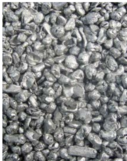
Aluminum shaped into balls in the rotor impact mill (RPMV)
