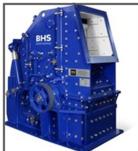
**Impact Crusher and Impact Mill (PB/PM)**: These units are a universal and economical solution. Both the impact crusher and impact mill achieve a very high crushing ratio with a constant grain-size curve for a broad range of material. The units have a very large feed opening relative to their size which enables optimum utilization of the crushing chamber during the process sequence and prevents clogging.
