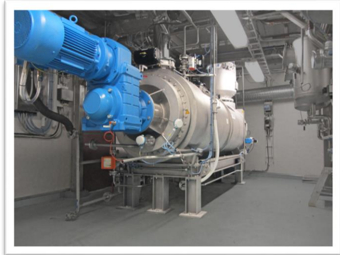
AVA Continuous Horizontal Vacuum Dryer Model HTK-T-1700 Steam-heated shaft and double-jacket
