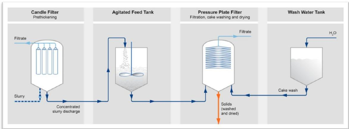
**Figure 4: MEG Process Flow for BHS Combination System**
