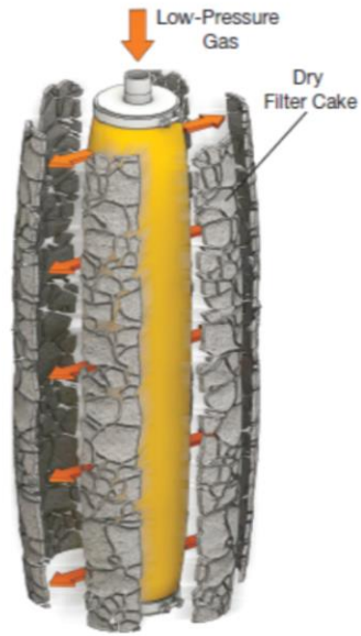
▲ Figure 3. During discharge, gas is fed into the top of the candle, which expands the flexible filter sock. This causes the dry cake to crack and break away from the filter. The solids are collected at the bottom of the pressure vessel.
