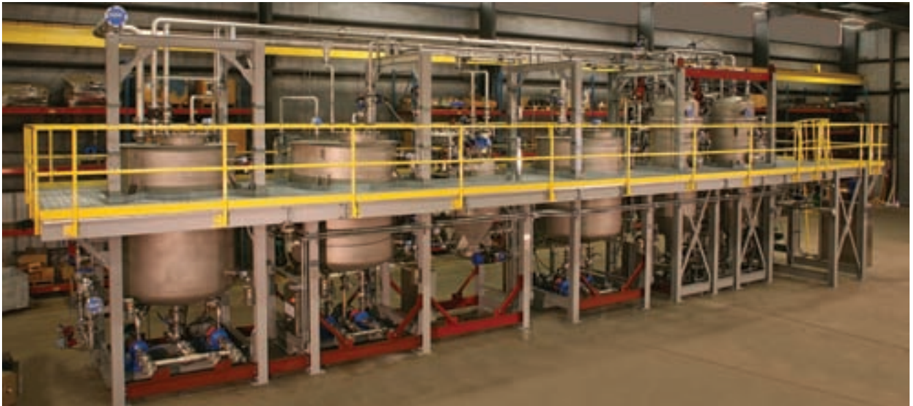
Figure 3 Amine application showing BHS combination of concentrating candle filters and pressure plate filters
