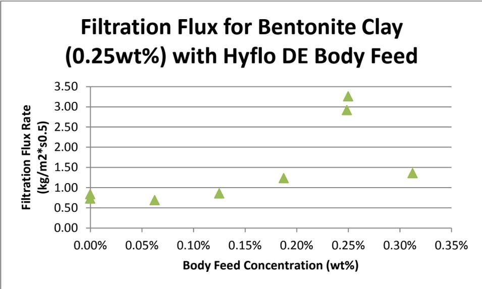
**Figure 8:** Average filtration flux rate for bentonite clay (0.25 wt.%) with various concentrations of Hyflo DE at 30psig filtration pressure
