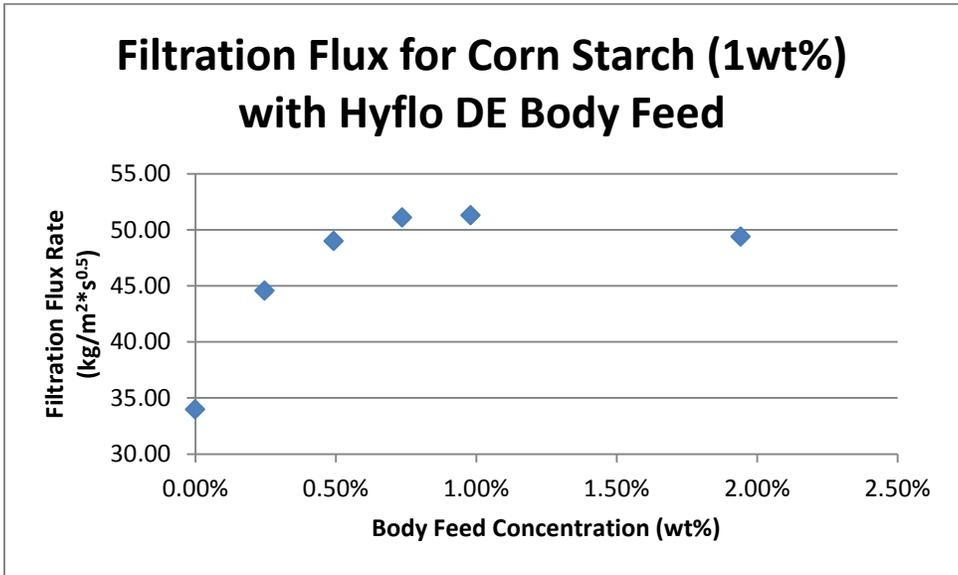
**Figure 6:** Average filtration flux rate for corn starch (1 wt.%) with various concentrations of Hyflo DE at 30 psig filtration pressure
