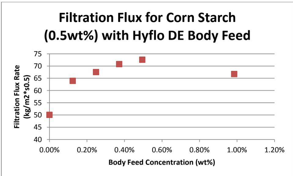
**Figure 7:** Average filtration flux rate for corn starch (0.5wt%) with various concentrations of Hyflo DE at 30psig filtration pressure
