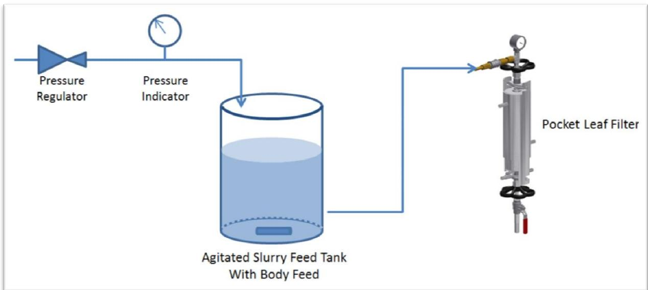
**Figure 4:** Filtration test setup diagram
