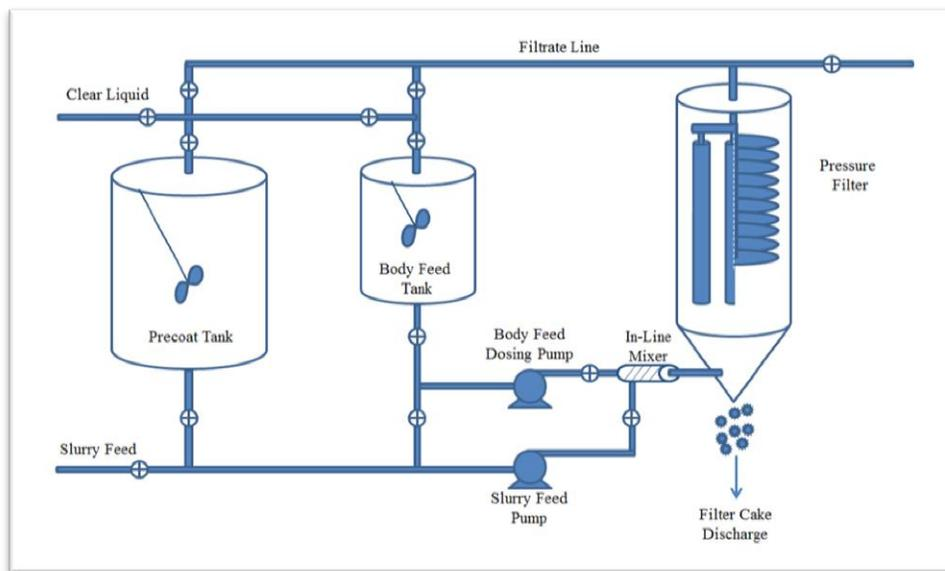
**Figure 1:** Process flow diagram for precoat and body feed processes with filter aid and filtration via candle or plate filter (Sentmanat, 2011)
