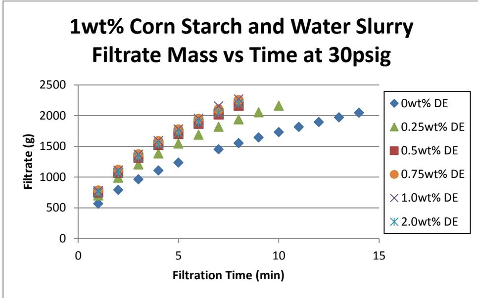
**Figure 5:** Filtration results for corn starch and water filtration with Hyflo DE body feed at various concentrations
