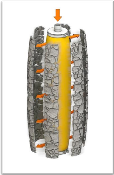
Figure 3: Candle Filter Cake Discharge
