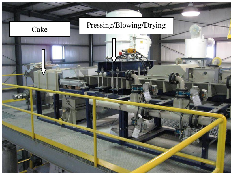
Figure 6: Cake Discharge End & Pressing/Blowing/Drying Device
