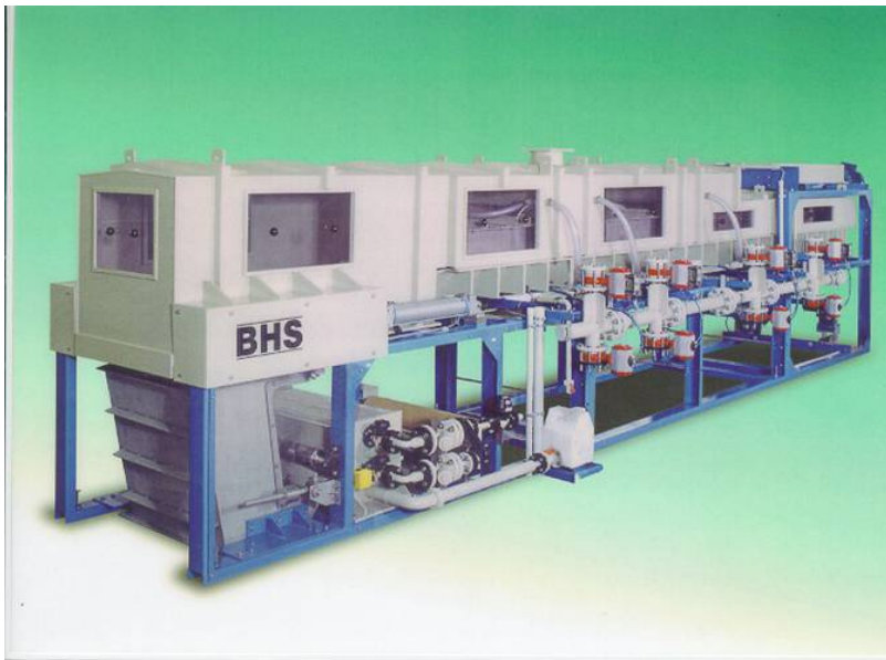
Figure 6: BHS Vacuum Belt Filter with Polypropylene Cover (Box-Design)
