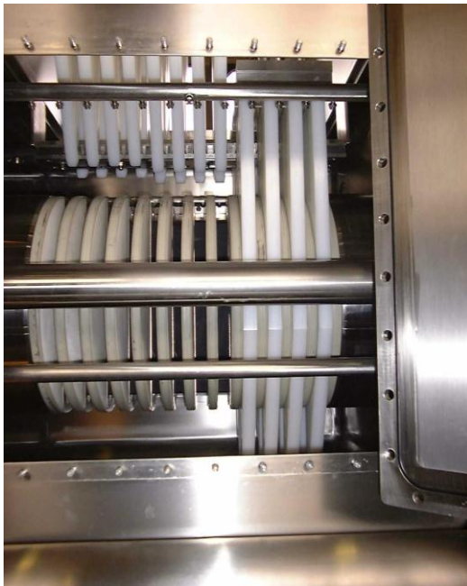
Figure 10: Elastomeric knives sequentially and automatically discharge the circular cakes
