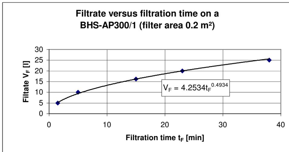
**Figure 1: Example of a Typical Filtration Curve**
