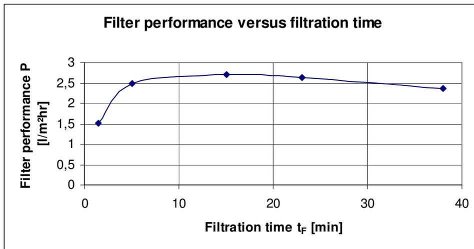
From the curve, for this example, the maximum filter performance is obtained when the filtration time of 15 minutes equals the side time of 15 minutes. The mathematical formulas follow on page 4 of this article.
