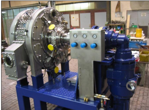
Figure 4: BHS Rotary Pressure Filter, RPF 0.18 M 2 , Pilot Filter
