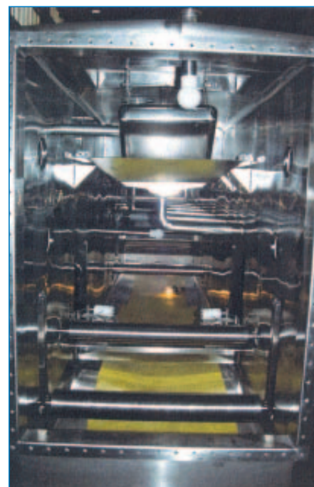
Figure 6 – Internal design with spray balls and fully drainable surfaces
