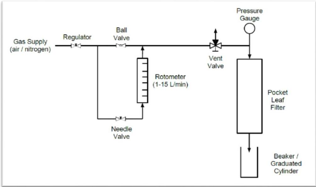
**Figure 7: BHS Pocket Leaf Filter for Pressure Testing**
