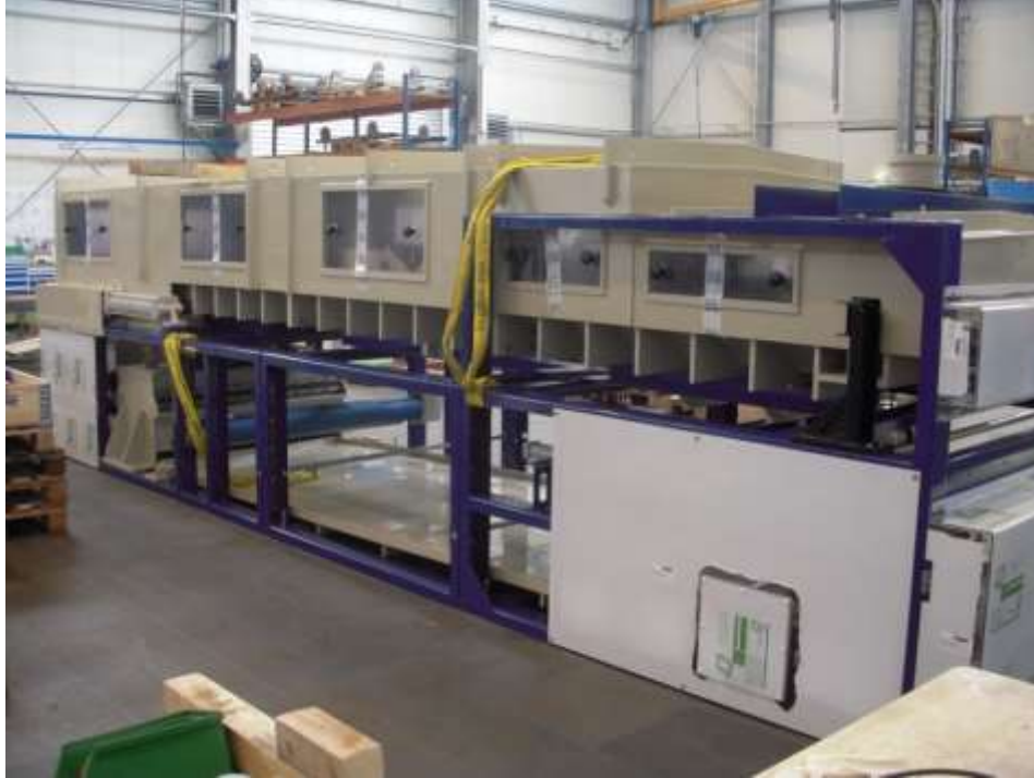
Image 2. Polypropylene belt filter with fume hood built for the filtration, washing, and drying of the sulfuric acid slurry.
