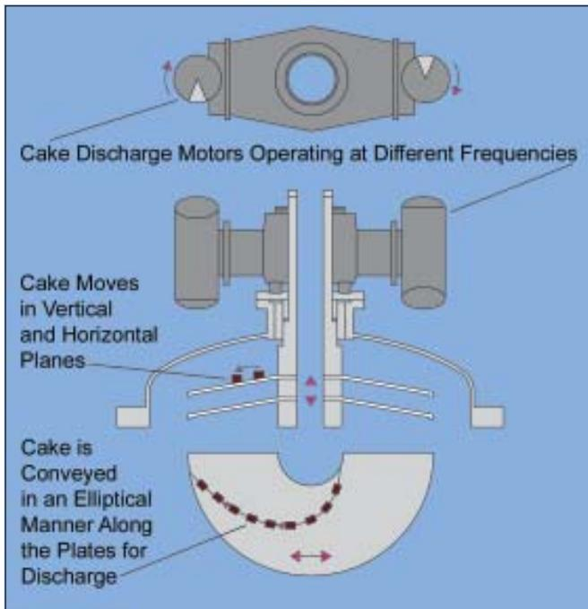
Figure 5. Cake discharge in the pressure plate filter.
