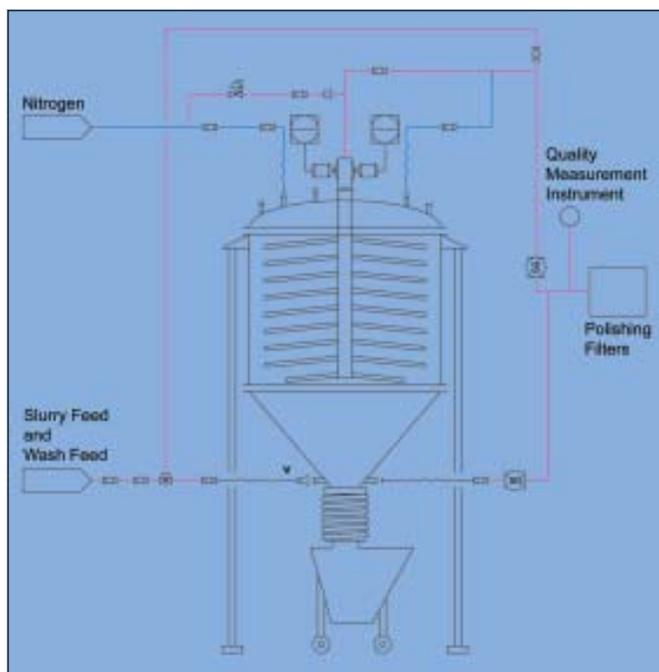
Figure 10. BHS pressure plate filter for cGMP production.
