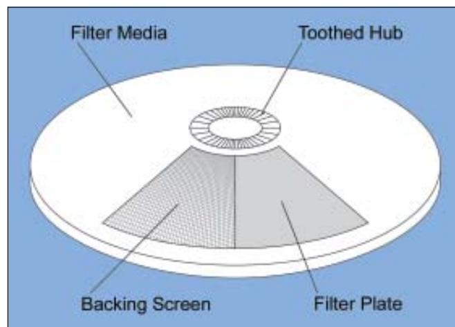
Figure 4. Filter plate.
