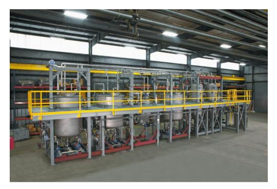
Figure 2: Amine Application Showing BHS Combination of Concentrating Candle Filters and Pressure Plate Filters
