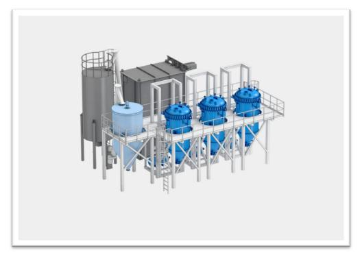
Figure 1: Conventional Single-Step Precoat Filtration
