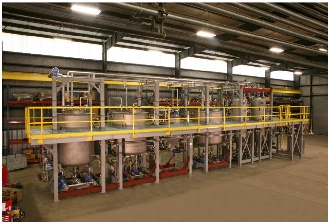
Figure 8: Complete Skid Package with Candle Filters, Plate Filter, Tanks, Pumps and PLC Controls
