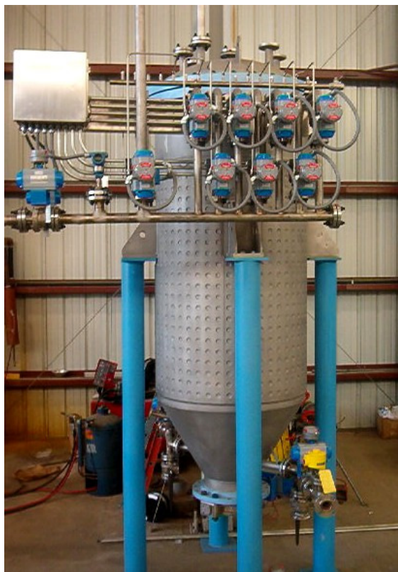
Figure 7: Jacketed Candle Filter with Register-Filtrate Piping & Junction Box
