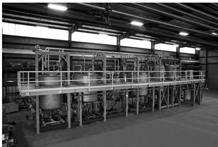
Fig 8: Complete skid package with candle filters, plate filter, tanks, pumps and PLC controls
