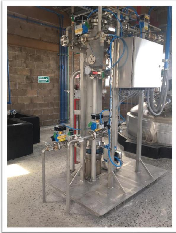
**Figure 9: BHS Pharma Candle Filter for Concentrated Slurry Discharge**
