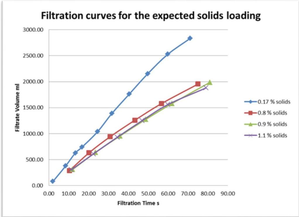
**Figure 8: BHS Process Filtration Curves**
