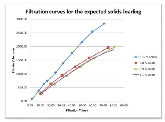
Figure 8: BHS Process Filtration Curves
