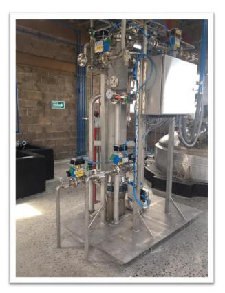
Figure 9: BHS Pharma Candle Filter for Concentrated Slurry Discharge
