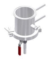
Put the clamp around the bottom and intermediate section to lock the components together.
